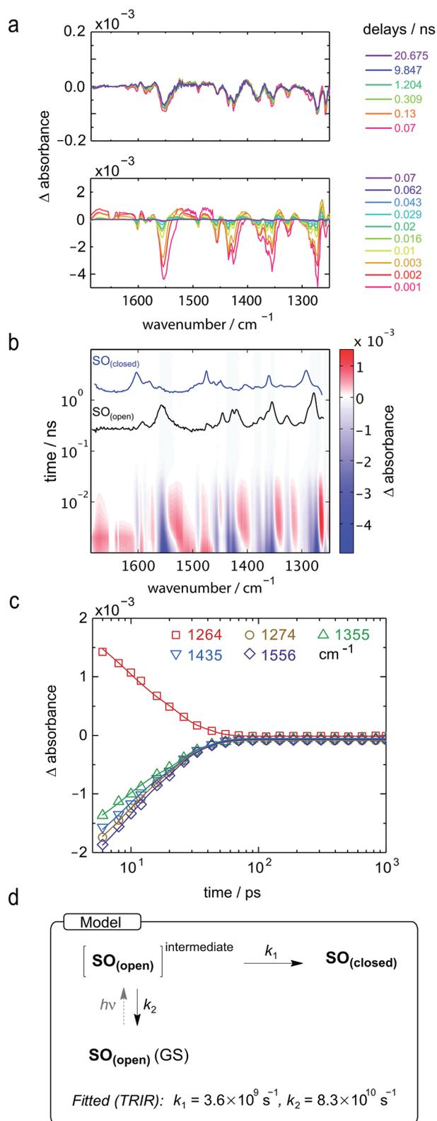
Fig. 6 TRIR spectra and excited-state kinetics of the ring-closing process of  $\text{SO}_{(\text{open})}$  in  $\text{CD}_2\text{Cl}_2$  by excitation at 590 nm. (a) TRIR spectra for selected probe times. (b) TRIR contour spectra; the steady-state spectra are shown for reference. (c) Kinetic traces for selected wavenumbers (points) and fitted kinetics (solid lines) using the values obtained from target analysis. (d) Model used to fit the TRIR. Laser energy: 800 nJ.
