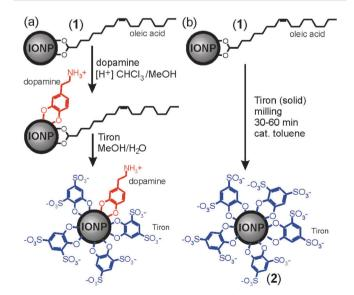
**Scheme 1** Synthesis of water-soluble IONPs by: (a) two-step ligand exchange in solution, leading to exchange of oleic acid ligands  $^{13}$  and (b) herein demonstrated one-step mechanochemical solvent-free process.
