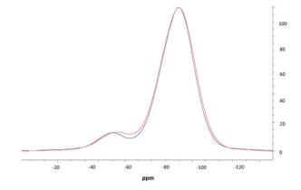
**Fig. 4** The CPMAS NMR spectra of thiolated silica (blue) and PEOZylated silica (red).
