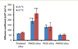
Fig. 6 Diffusion coefficients for thiolated, and POZylated silica nanoparticles through a 1% gastric mucin dispersion at 25 and 37 °C. Error bars represent the mean  $\pm$  standard deviation of 3 repeats.
