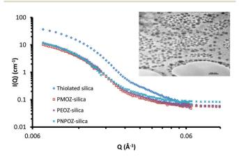
**Fig. 5** SANS profiles for thiolated silica (blue), PMOZ-silica (red), PEOZ-silica (green), and PNPOZ-silica (purple) nanoparticles. The insert shows the TEM image for unfunctionalised thiolated silica, used for the fitting. The scale-bar represents 100 nm.
