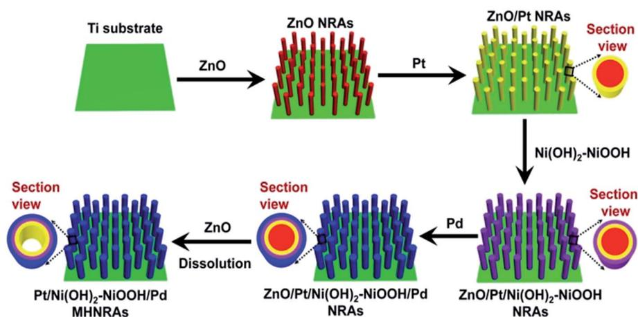
Scheme 1 Fabrication of the Pt/Ni(OH)<sub>2</sub>-NiOOH/Pd MHNRA.
