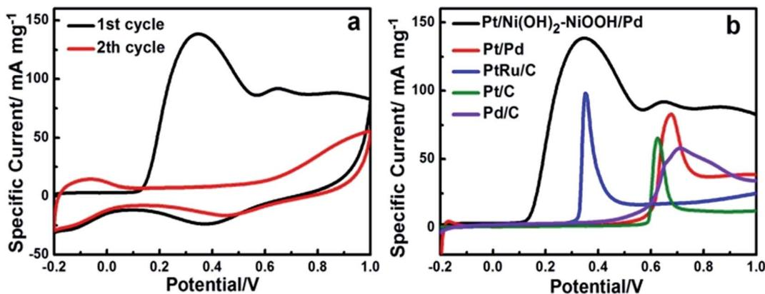
Fig. 4 (a) CO stripping voltammograms on the Pt/Ni(OH)<sub>2</sub>-NiOOH/Pd MHNRA performed in a solution of 0.5 M H<sub>2</sub>SO<sub>4</sub> at 20 mV s<sup>-1</sup>; (b) the comparison of the CO stripping voltammograms of the Pt/Ni(OH)<sub>2</sub>-NiOOH/Pd MHNRA, Pt/Pd MHNRA, commercial Pt/C, Pd/C and PtRu/C catalysts.
