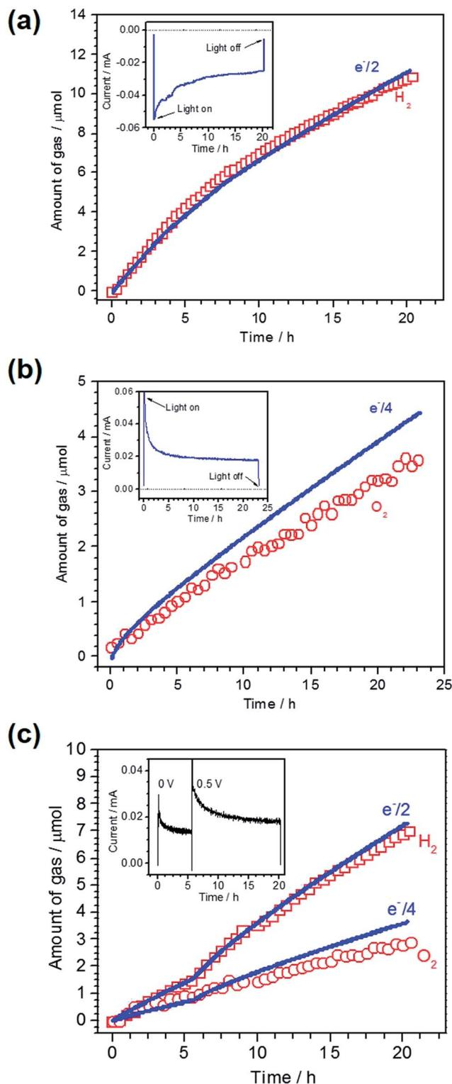
Fig. 2 Evolution of hydrogen/oxygen from the two-electrode system under visible light ( $\lambda > 420$  nm) irradiation. (a) Pt/LTC/Au ( $3.5 \text{ cm}^2$ ) – Pt wire under a bias of  $-0.9$  V, (b) CoPi/LTC/Ti ( $4.3 \text{ cm}^2$ ) – Pt wire under a bias of  $0.8$  V and (c) CoPi/LTC/Ti ( $4.5 \text{ cm}^2$ ) – Pt/LTC/Au ( $2 \text{ cm}^2$ ) under a bias of  $0$  and  $0.5$  V. The inset shows current–time curves recorded during the respective measurements.
