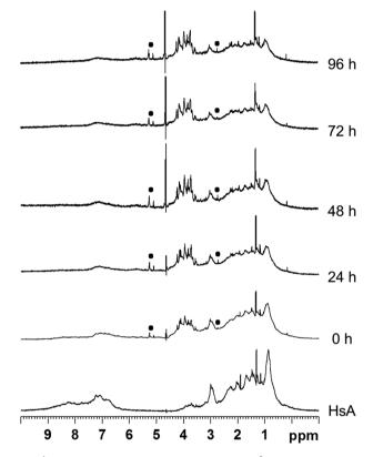
**Fig. 2** <sup>1</sup>H NMR spectra of the mixture HsA/ $[1]^{6+}$  (molar ratio 1:10) recorded in D<sub>2</sub>O at 37 °C between 0 h and 96 h. The <sup>1</sup>H NMR spectrum of free HsA is shown at the bottom as reference. The *p*-cymene resonances of the metallaprism are labelled by (**m**).
