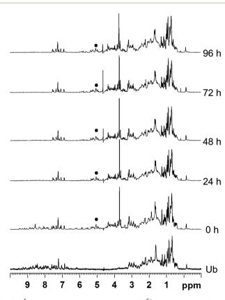
**Fig. 3** <sup>1</sup>H NMR spectra of the mixture Ub/ $[1]^{6+}$  (molar ratio 1:10, D<sub>2</sub>O, 37 °C) recorded between 0 h and 96 h. The <sup>1</sup>H NMR spectrum of free ubiquitin is shown as reference at the bottom. The *p*-cymene resonances of the metallaprism are labelled by (**■**).
