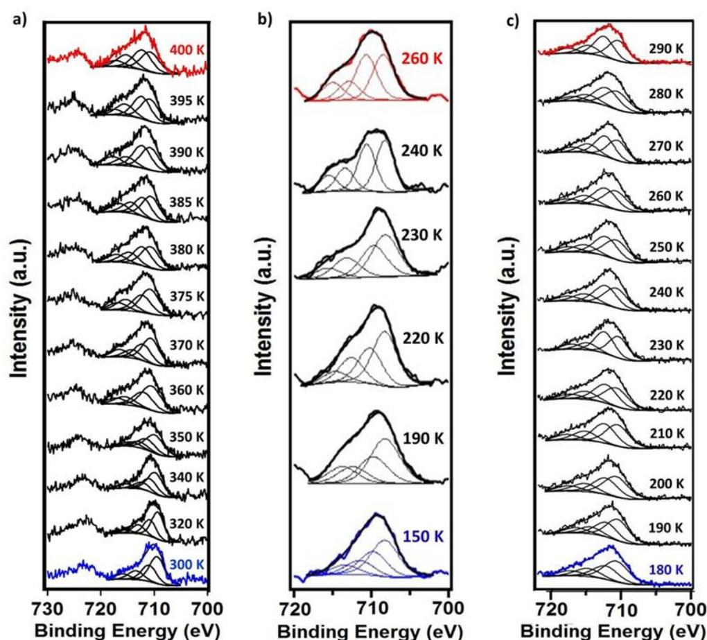
Figure 3: Temperature-dependent X-ray photoemission spectra of a) **1**- [Fe(L1)(bipy)]<sub>n</sub>, b) **2**- [Fe(L2)(bipy)]<sub>n</sub>, and c) **3**- [Fe(L3)(bpee)]<sub>n</sub>. The spectrum in red is representative of the high spin state while the spectrum in blue is representative of the low spin state.
