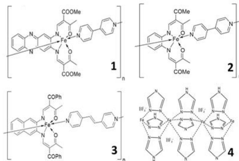
Figure 1: A schematic representation of spin crossover coordination polymers discussed in this work: 1-  $[\text{Fe}(\text{L1})(\text{bipy})]_n$ , 2-  $[\text{Fe}(\text{L2})(\text{bipy})]_n$ , 3-  $[\text{Fe}(\text{L3})(\text{bpee})]_n$  and 4-  $[\text{Fe}(\text{Htrz})_2(\text{trz})](\text{BF}_4)$ .
