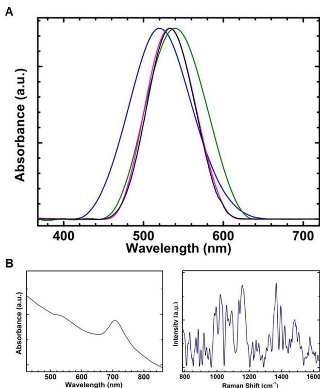
**Figure 2.** A) Spectral behavior of 3 nm gold nanoparticles (blue), gold arrays (green), AuSi3 (purple), and calcinated AuSi3 (black). Spectra were collected in milliQ water, normalized and the background subtracted. B) Absorbance (left) and SERS (right, background subtracted) spectra of AuSi3A collected, respectively, in ethanol and milliQ water.
