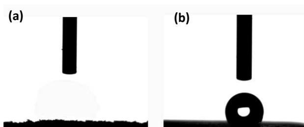
**Fig. 4** Contact angle tests for water of TiO<sub>2</sub> aerogels before (a) and after (b) modified by TEOS
