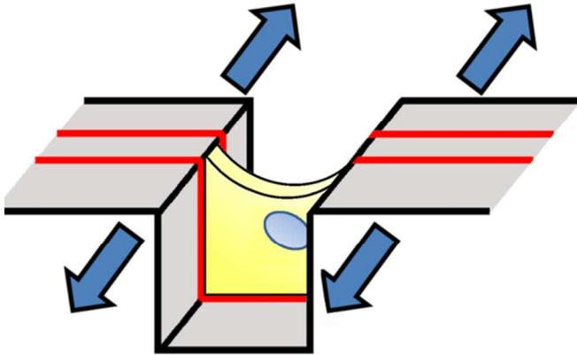
We develop a technique to generate well-defined adhesive micropatterns on topologically complex substrates, enabling the culture of individual cells in precisely-controlled, three-dimensional adhesive microstructures.
