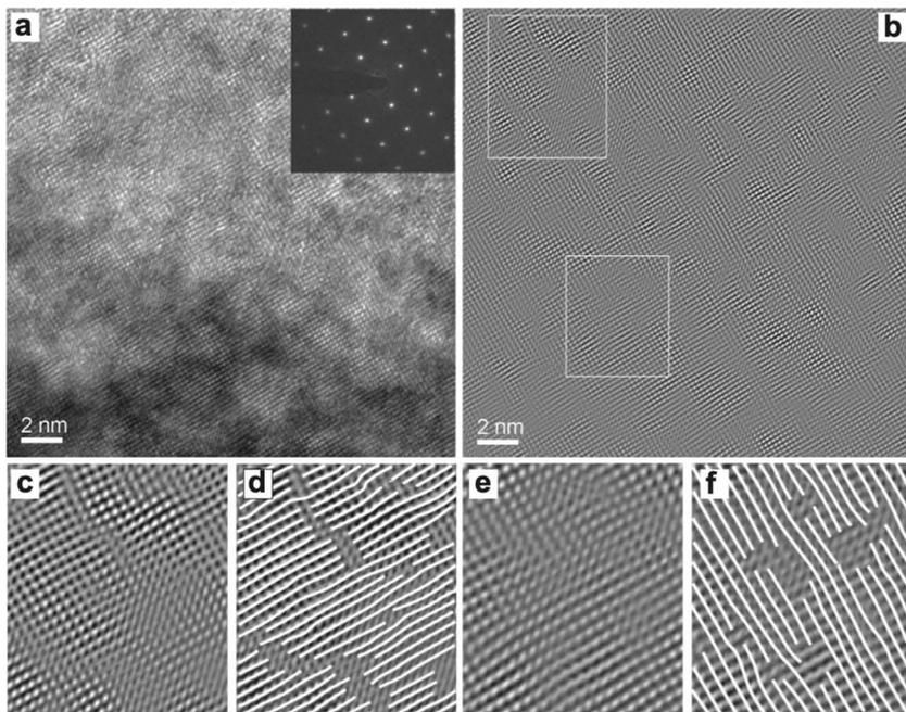
**Fig. 11** HRTEM images of the equiatomic quaternary NbMoTaW bcc Senkov alloy: (a) bright-field (BF) image with [100] zone axis; (b) corresponding inverse fast-Fourier transform; (c) and (e) enlarged images of the boxes in (b); and (d) and (f) traces corresponding to (c) and (e) to show the lattice distortions (after Zou *et al.*<sup>57</sup>). Reproduced with permission from Elsevier from ref. 57.
