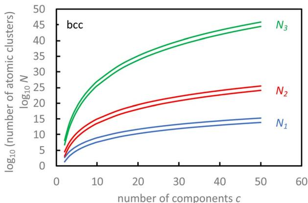
Fig. 10 Number of different oriented (upper lines) and non-oriented (lower lines) local atomic clusters out to first ( $N_1$ ), second ( $N_2$ ) and third ( $N_3$ ) near neighbours for a multi-component single-phase bcc material with  $c$  components.
