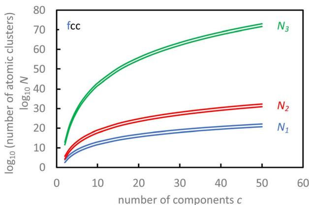
**Fig. 9** Number of different oriented (upper lines) and non-oriented (lower lines) local atomic clusters out to first ( $N_1$ ), second ( $N_2$ ) and third ( $N_3$ ) near neighbours for a multicomponent single-phase fcc material with  $c$  components.
