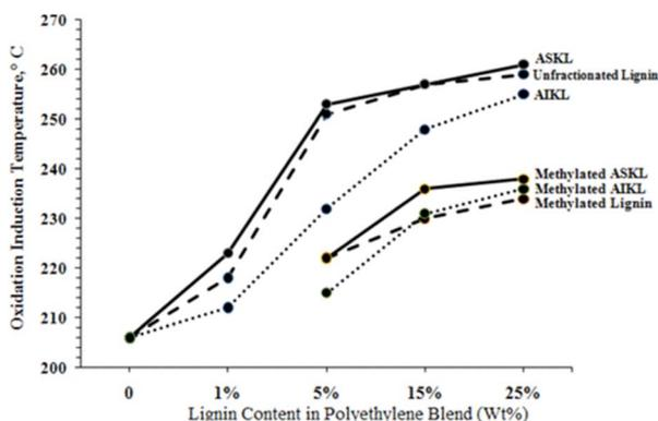
Fig. 14 Correlation of lignin content (unfractionated SKL and its fractions) in PE-blends with  $OI_{temp}$ . Reproduced from ref. 168 with permission from the American Chemical Society, copyright 2015.
