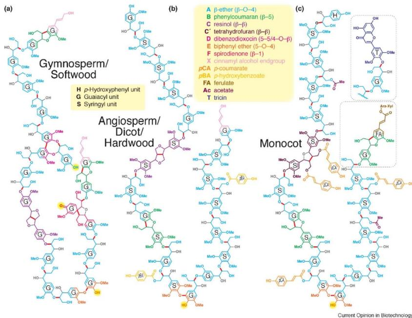
Fig. 1 Current lignin structure according to Ralph, Lapierre, and Boerjan.<sup>4</sup> Reproduced from ref. 4 with permission from Elsevier, copyright 2019.
