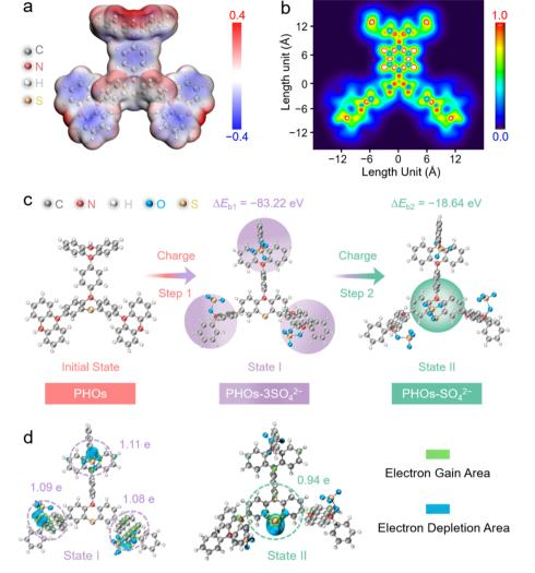
Fig. 4 Theoretical simulations of redox processes of PHOs at various electrochemical states. (a) MEP distribution. (b) ELF- $\pi$  map. (c) Optimized geometries and corresponding  $\Delta E_D$  values after ion coordination. (d) Differential charge isosurfaces at state I and II.
