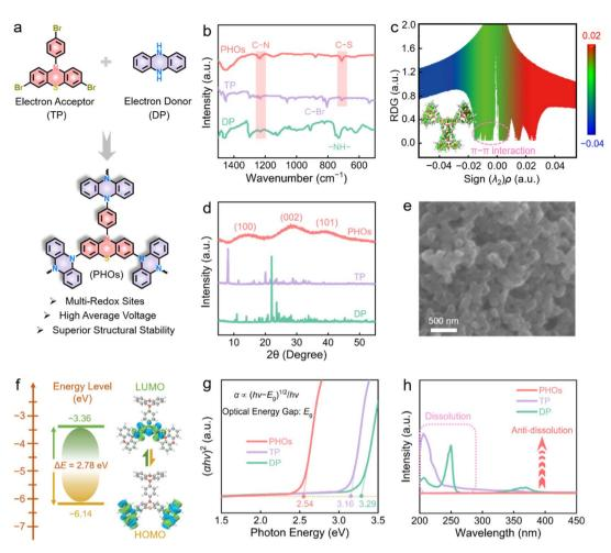
Fig. 1 Structural characterization of PHOs. (a) Synthetic route for PHOs. (b) FT-IR spectra and (c) scatter plots of RDG against sign( $\lambda_2$ ) $\rho$  and the gradient isosurface. (d) XRD pattern. (e) SEM pattern. (f) Energy levels and frontier molecular orbitals. (g) Calculated  $E_g$  values. (h) UV/Vis spectra of aqueous ZnSO $_4$  solution soaked with TP, DP and PHOs for three months.
