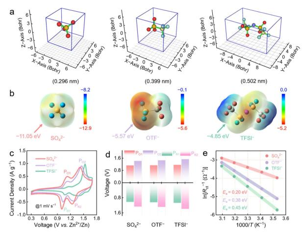
Fig. 2 Electrochemical behavior of PHOs in different electrolytes. (a) Anion size. (b) ESP of the anions. (c) CV curves. (d) Redox peak position. (e) Calculated  $E_a$  values of PHOs in  $SO_4^{2-}$ , OTF<sup>-</sup>, and TFSI<sup>-</sup> based electrolytes
