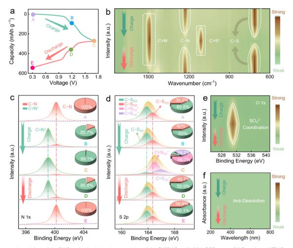
Fig. 5 Structural evolution of the PHO cathode during the operation of the Zn $\parallel$ PHOs cell. (a) A GCD curve. (b) Overview of FT-IR spectra. XPS spectra of (c) N 1s, (d) S 2p, and (e) O 1s at various electrochemical states. (f) UV-vis spectra and photographs of aqueous ZnSO<sub>4</sub> electrolyte during (dis)charging.
