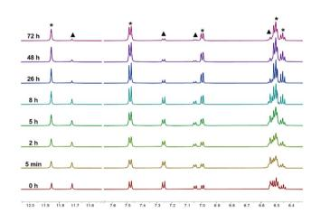
Fig. 2  $^{1}$ H NMR spectrum (600 MHz, DMSO- $d_{6}$ , 298 K) of the transformation of Na<sub>4</sub>[Si<sub>2</sub>D<sub>3</sub>] from helicates ( $\Lambda\Lambda/\Delta\Delta$ ) to mesocate ( $\Lambda\Delta$ ) over time. ( $\Delta$  represents helicates ( $\Lambda\Lambda/\Delta\Delta$ ) and \* represents mesocate ( $\Lambda\Delta$ )).
