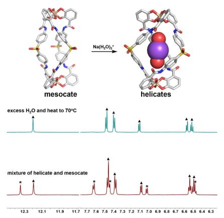
Fig. 4 Comparison of  $^1$ H NMR spectra (600 MHz, DMSO- $d_6$ , and 298 K) of mixtures of  $Na_4[Si_2E_3]$  isomers before and after heating with excess  $H_2O$  at 70 °C. ( $\blacktriangle$  represents helicates ( $\Lambda\Lambda/\Delta\Delta$ ) and \* represents mesocate ( $\Lambda\Delta$ )).
