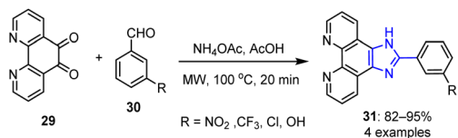
Scheme 7 Synthesis of imidazo[4,5- f ]-1,10-phenanthroline derivatives 31 under MW irradiation.
