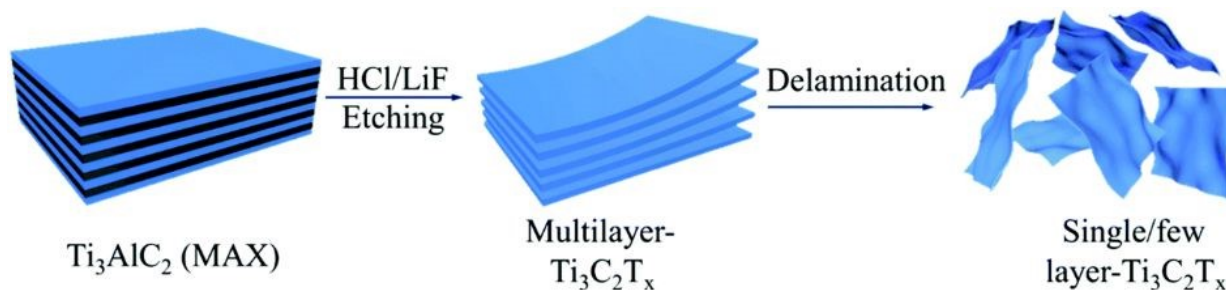
Figure 5: Scheme of the fabrication procedure of MXene. This figure has been reproduced from ref [142] with permission from Journal of Materials Chemistry C, copyright 2019.
