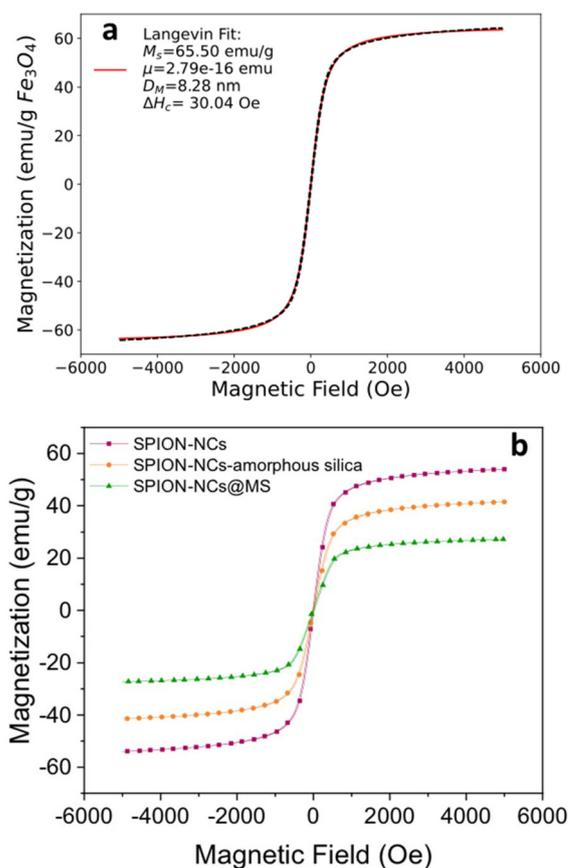
Fig. 5 Magnetization curves of (a) the SPION-NCs normalized to the weight of  $\text{Fe}_3\text{O}_4$  and (b) the SPION-NCs alone and after coating with amorphous silica, followed by mesoporous silica (MS) normalized to overall sample weight.
