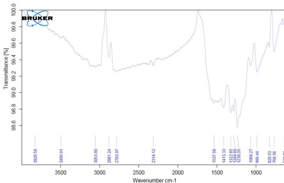
Fig. 9 FT-IR spectrum of the reused BCNSA catalyst after the 6<sup>th</sup> cycle.
