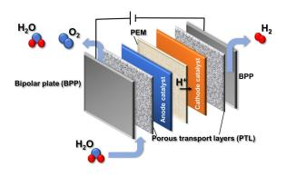
Figure 1 Illustration of a single cell used in PEM water electrolysis.
