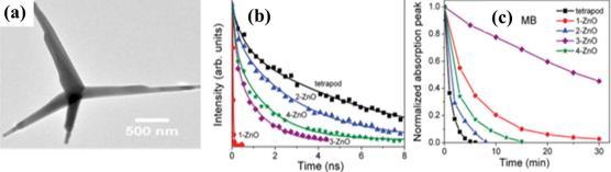
Fig. 14 (a) SEM image of ZnO TPs (b) PL decay curves and (c) degradation curve for MB dye for various ZnO nanostructures. (Reprinted with permission from ref. 45 Copyright 2011, American Chemical Society].
