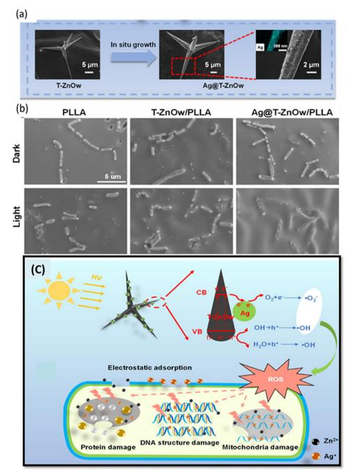
Fig. 12 (a) In situ growth of ZnO/TPw (b) different morphologies of E coli cells (c) diagram showing the Ag@T-ZnOw/PLLA scaffolds antibacterial action when exposed to visible light. [Reprinted with permission from ref. 100 Copyright 2022, Elsevier].
