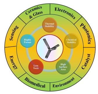
Fig. 4 Various properties and applications of ZnO TPs
