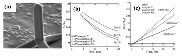
Fig. 9 (a) SEM image of ZnO TPs (b) curves of the photocatalytic degradation of MO under UV-vis, visible, and direct solar light and (c) determination of the reaction rate constant (k, min<sup>-1</sup>) [Reprinted with permission from ref. 79 Copyright 2023, Springer Nature].
