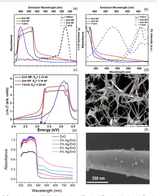
Fig. 5 For various ZnO nanostructures- (a) and (b) UV-visible absorption and PL spectra, (c) The estimated bandgap using Tauc plot. (d) SEM image of ZnO TPs. <sup>55</sup> (e) UV-vis DRS Spectra of ZnO TPs and Ag/ZnO TPs (with Ag 2%, 3%, 4% and 5%) [Reprinted with permission from ref. 56 Copyright 2017, Elsevier] (f) SEM image of 4% Ag/ZnO TPs [Reprinted with permission from ref. 56 Copyright 2017, Elsevier].
