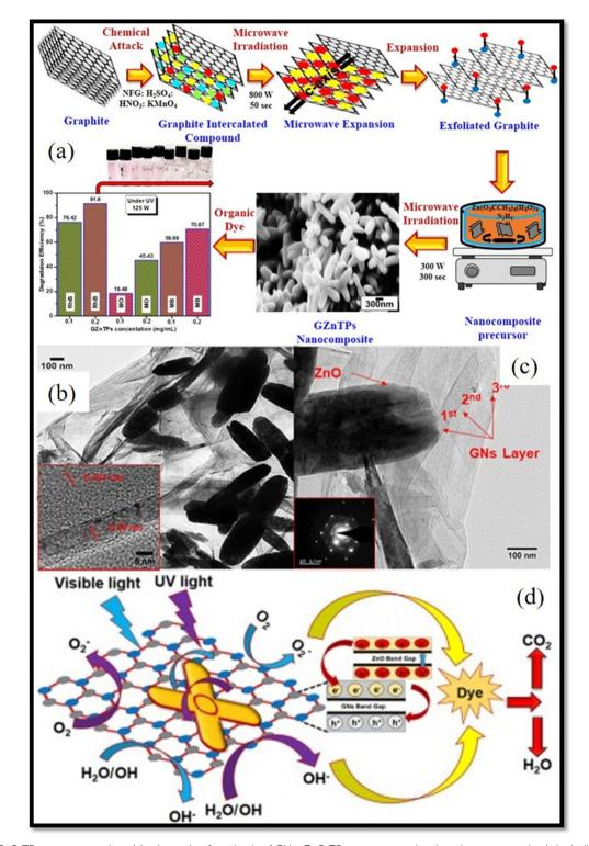
Fig. 11 GNs-ZnO TPs nanocomposites: (a) schematic of synthesis of GNs-ZnO TPs nanocomposites by microwave synthesis including SEM image of nanocomposites (b) and (c) HRTEM and (d) photocatalytic mechanism of GNs-ZnO TPs nanocomposites. [Reprinted with permission from ref. 84 Copyright 2021, Elsevier].
