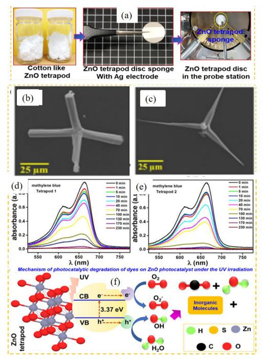
Fig. 10 (a) Preparation of ZnO TPs based sponge, (b) and (c) ZnO TPs with different arm sizes as TP1 and TP2 respectively. Photodegradation activities of (d) TP1 and (e) TP2 under UV light irradiation for MB dye solution and (f) Mechanism of photocatalytic degradation using TP sponge.<sup>25</sup>
