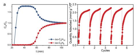
Fig. 4 (a) Breakthrough experiment on ZU-603 using a gas mixture of iso- $C_4H_8/i$ so- $C_4H_{10}$  (50/50, v/v) with a mix gas flow rate of 0.8 mL min<sup>-1</sup> at 298 K and (b) cycling adsorption tests of iso-C<sub>4</sub>H<sub>8</sub> on ZU-603 at 298 K.
