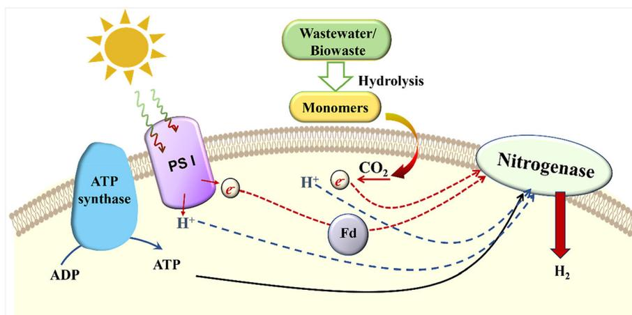
Fig. 2 Mechanism diagram of photo-fermentative biohydrogen production.
