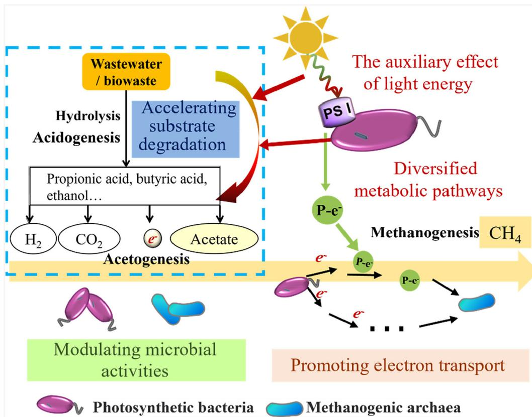
Fig. 4 Mechanism diagram of photo-fermentative biomethane production.
