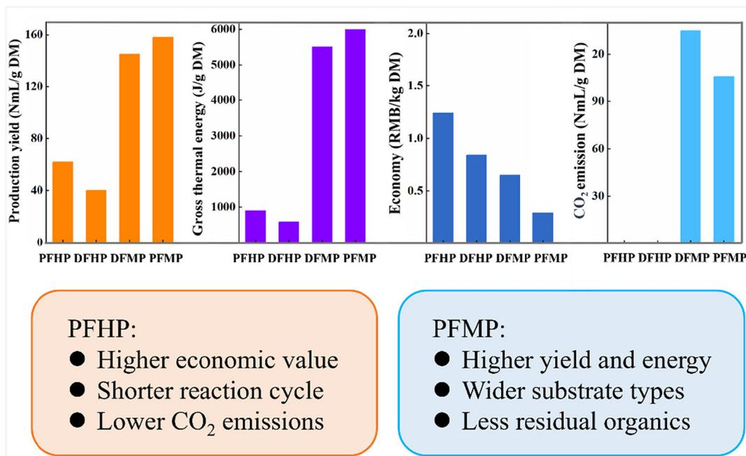
**Fig. 5** Comprehensive analysis of biohydrogen and biomethane produced from photo-fermentation systems. PFHP represents photo-fermentative hydrogen production. DFHP represents dark-fermentative hydrogen production. DFMP represents photo-fermentative methane production. PFMP represents photo-fermentative methane production.
