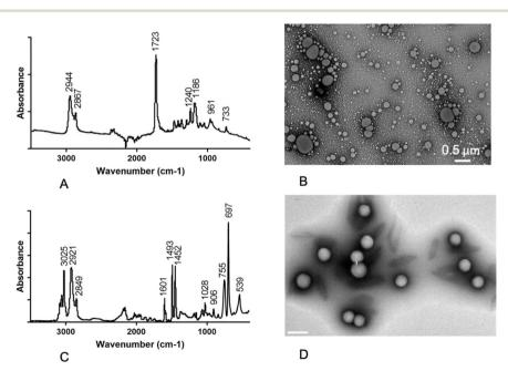
Fig. 1 Characterization of the plastic beads. Chemical characterization of the PCL and PS beads was carried out by FT-IR spectroscopy (panels A and C, respectively). Physical characterization of the beads was carried out by transmission electron microscopy (panels B and D, respectively).
