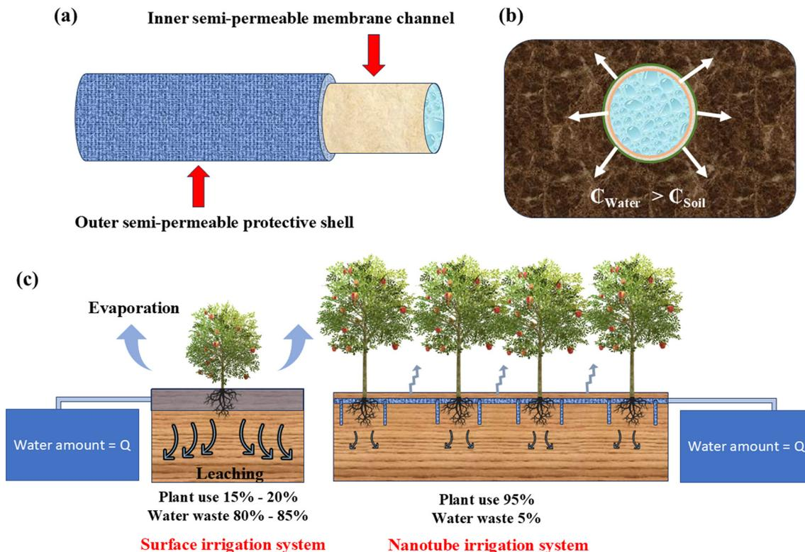
Fig. 5 (a) Internal structure of Moistube,<sup>169</sup> (b) water flow from Moistube to the surrounding soil, depending on soil water potential, and (c) irrigation water use efficiency of Moistube compared to the conventional surface drip irrigation system.
