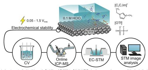
Fig. 1 Electrochemical system studied in this work. Stability of Pt(111) in 0.1 M HClO<sub>4</sub> in absence and presence of the ionic liquid [C<sub>2</sub>C<sub>1</sub>Im][OTf]. We probe the electrochemical stability of the system applying CV, online ICP-MS, EC-STM and using an algorithmic pattern recognition approach to analyze STM images
