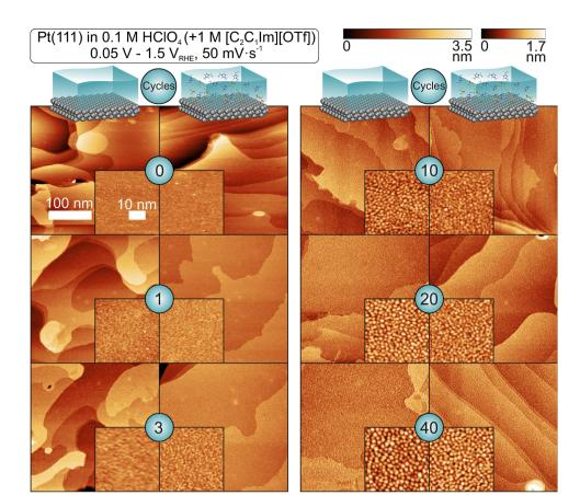
Fig. 4 EC-STM images ( $U_{\text{bias}}$  0.4 V,  $I_{\text{t}}$  0.2-1 nA) before and after the initial oxidation-reduction cycles (0.05-1.5  $V_{\text{RHE}}$ , 50 mV s<sup>-1</sup>) in the absence (left) and presence (right) of 1 M [C<sub>2</sub>C<sub>1</sub>Im][OTf]. Supporting electrolyte was 0.1 M HClO<sub>4</sub>.
