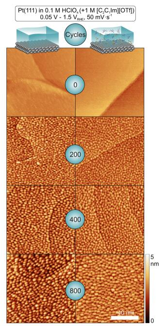
Fig. 5 EC-STM images ( $U_{\rm bias}$  0.4 V,  $I_{\rm t}$  0.2–1 nA) after extended ORCs (0.05-1.5 V<sub>RHF</sub>, 400 mV s<sup>-1</sup>) in the absence (left) and presence (right) of 1 M [C<sub>2</sub>C<sub>1</sub>Im][OTf]. Supporting electrolyte was 0.1 M HClO<sub>4</sub>.
