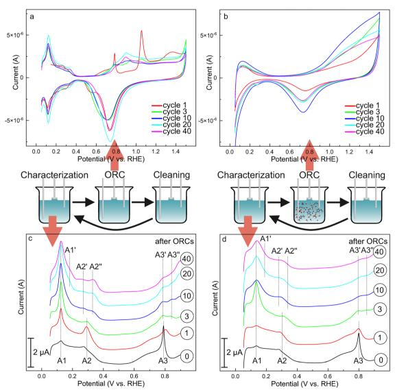
$\textbf{Fig. 2} \quad \textbf{Cyclic voltammograms of Pt(111) during ORCs (0.05-1.5 \ V_{RHE}, 50 \ \text{mV s}^{-1}) in the absence (a) and presence (b) of 1 \ M \ [C_2C_1Im][OTf]. \ Corresponding and the large of the$ characterization CVs (0.05-0.9 V<sub>RHE</sub>, 50 mV s<sup>-1</sup>) measured after ORCs in absence (c) and presence (d) of IL in blank electrolyte only (0.1 M HClO<sub>4</sub>). An additional cleaning step was performed between the ORCs and the characterization.
