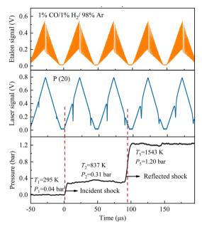
Fig. 7 Raw data of laser signal, etalon signal, and pressure measured in the shock tube.
