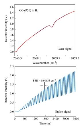
Raw data of laser signal and etalon signal measured in the gas cell.
