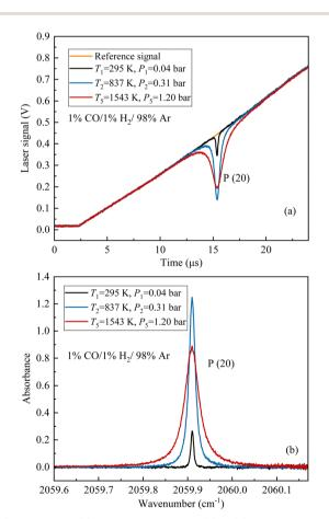
Fig. 8 Laser signal (a) and measured spectra (b) of CO at different status in the shock tube.
