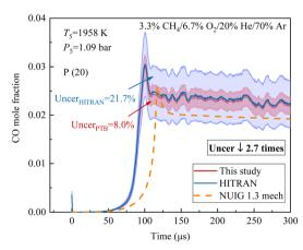
Fig. 12 Time-resolved CO mole fraction of CH<sub>4</sub> oxidation measured in the shock tube and calculated using NUIG 1.3 mechanism.<sup>40</sup>
