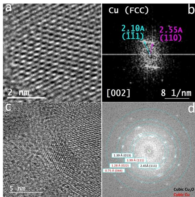
**Fig. 10** Upper panel for the glass-exchanged sample: HRTEM image (a) and its crystallographically analysed fast Fourier transform [FFT] result, revealing the [002] plane of the cubic crystal of copper (b); lower panel for the glass-exchanged sample, 10<sup>6</sup> Gy irradiated and annealed at 600 °C for 60 minutes: HRTEM image (c) and its crystallographically analysed FFT result (d), revealing the fingerprints of cubic copper (red) and cubic Cu<sub>2</sub>O (black) crystals.
