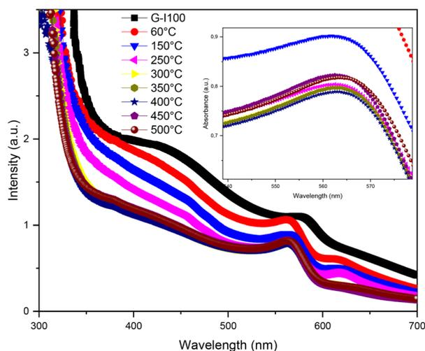
**Fig. 7** Optical absorption spectra for G-I100 before the annealing treatment and after annealing (G-IA100) at temperatures between 60 and 500 °C. The inset shows a magnification for the obtained spectra in the wavelength range between 540–580 nm.
