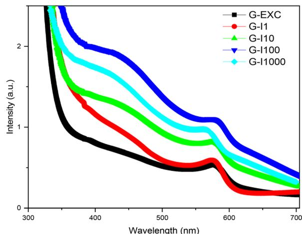
**Fig. 5** Optical absorption spectra for the Cu-exchanged (black curve) and the irradiated samples with doses of 1 kGy (G-I1, red curve), 10 kGy (G-I10, green curve), 100 kGy (G-I100, blue curve) and 1000 kGy (G-I1000, baby blue curve).
