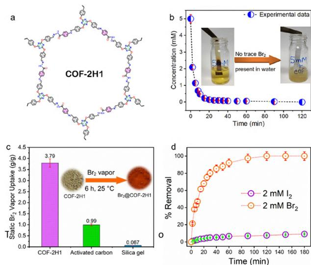
**Fig. 5** (a) Chemical structure of COF-2H1, (b) decreases in the concentration of bromine in water with time (inset: the KI starch paper test before and after bromine capture), (c) result of vapor phase static Br<sub>2</sub> uptake capacities, and (d) Br<sub>2</sub> and I<sub>2</sub> removal kinetics of COF-2H1 in cyclohexane. Reproduced with permission from ref. 28. Copyright 2024, American Chemical Society.
