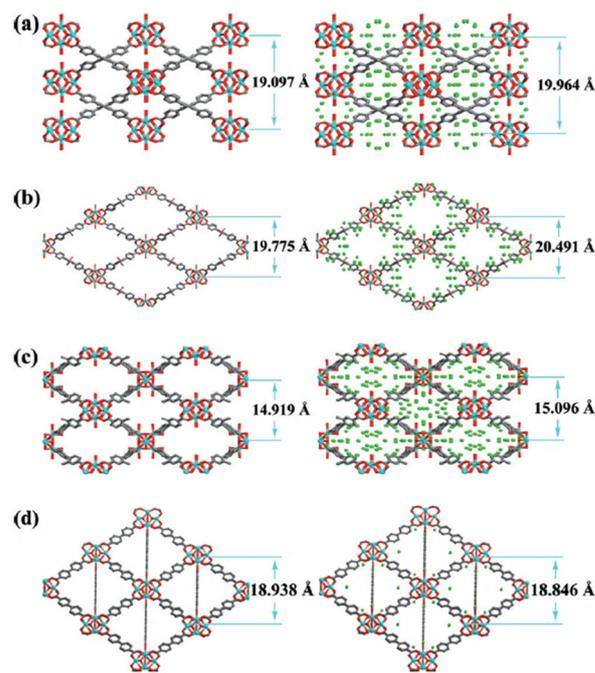
Fig. 2 The structures with their pore size of the MOFs: (a) PCN-605-H, (b) PCN-606-OMe, (c) PCN-700, and (d) UiO-67 before and after bromine adsorption. Reproduced with permission from ref. 23. Copyright 2017, Wiley-VCH Verlag GmbH & Co. KGaA, Weinheim.
