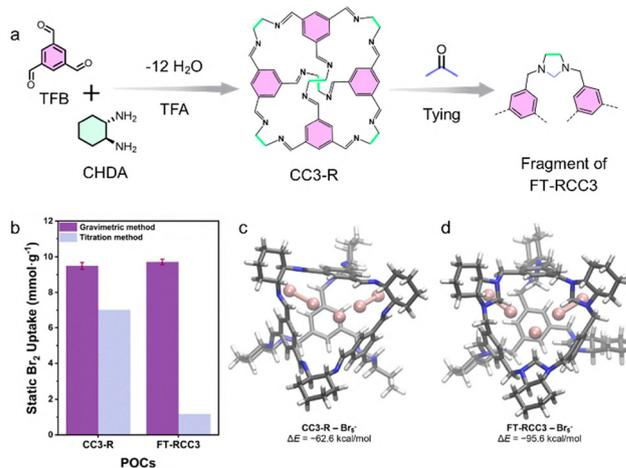
Fig. 7 (a) Schematic representation of the synthesis of CC3-R and FT-RCC3 porous organic cages. (b) Result of static Br<sub>2</sub> capture capacities of both the POCs determined through the gravimetric and titration methods. (c) and (d) DFT optimized structures and their corresponding binding energies of CC3-R and FT-RCC3, respectively with adsorbed polybromide Br<sub>5</sub><sup>-</sup>. Reproduced with permission from ref. 30. Copyright 2022, the Royal Society of Chemistry.
