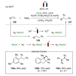
Fig. 24 Metal-catalyzed electrochemical diazidation of alkenes. Blue electrode: cathode; red electrode: anode
