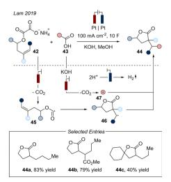
Fig. 9 Route towards substituted lactones by anodic generation of oxycarbonyl radicals. Blue electrode: cathode; red electrode: anode
