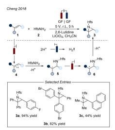
Fig. 2 Electrochemical aziridination by alkene activation using a sulfamate as the nitrogen source. HfsNH<sub>2</sub>; 1,1,1,3,3,3-hexafluoro-2-propyl sulfamate. GF: graphite felt; blue electrode: cathode; red electrode: anode.
