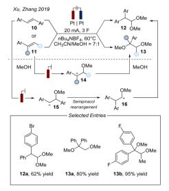
Fig. 4 Substrate-dependent electrochemical dimethoxylation of olefins. Blue electrode: cathode; red electrode: anode
