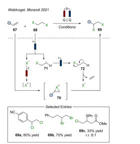
Fig. 14 Electrochemical dihalogenation of alkenes. Conditions: X = Br or X = Cl, SPh: 10 mA cm<sup>-2</sup>, 3–16 F, HFIP (1 vol%), Et<sub>4</sub>NBF<sub>4</sub> (0.2 M), r.t.,  $CH_3CN$ ,  $N_2$ . X = Cl: 4 mA cm<sup>-2</sup>, 2.5-9 F, MnCl<sub>2</sub>·4H<sub>2</sub>O (5 mol%),  $Et_4NBF_4$ (0.1 M), 50 °C, CH<sub>3</sub>CN, N<sub>2</sub>. Blue electrode: cathode; red electrode: anode.
