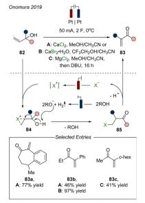
Fig. 17 Synthesis of  $\alpha$ -exo-methylene ketones from  $\alpha$ , $\alpha$ -disubstituted allyl alcohols by electrochemical oxidative migration. Blue electrode: cathode; red electrode: anode.
