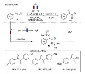
Fig. 5 Integrated electrochemical-chemical oxidation mediated by alkoxysulfonium ions. CF: carbon felt; blue electrode: cathode; red electrode: anode.
