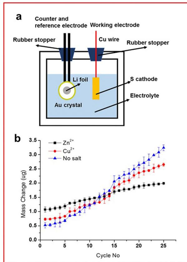
Fig. 15 (a) Schematic of an EQCM set-up for an LSB; (b) mass change measured through EQCM for the lithium anode with an electrolyte containing either no salt (blue) or TMA salt (Zn<sup>2+</sup> in black and Cu<sup>2+</sup> in red). ((a) and (b) Reproduced with permission from ref. 146, Copyright (2019) Elsevier.)
