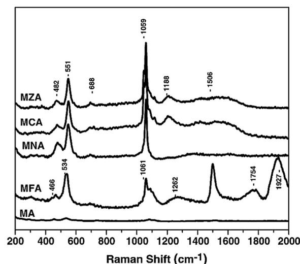
Fig. 8 Raman spectra of the different LDH samples.
