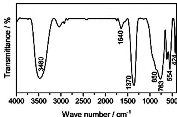
Fig. 5 FTIR spectra of ZnMgAl-LDHs (Zn/Mg = 0.125).
