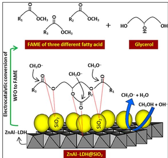
Fig. 10 Suggested mechanism of the transesterification process using the ZnAl/LDH-SiO<sub>2</sub> composite.
