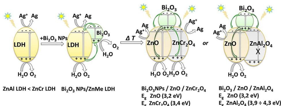
Scheme 4 Proposed mechanism for  $\text{O}_2$ -generation under solar-light irradiation over  $\text{Bi}_2\text{O}_3\text{NPs}/\text{ZnMe-LDH}$  and  $\text{Bi}_2\text{O}_3/\text{ZnO}/\text{ZnMe}_2\text{O}_4$ .
