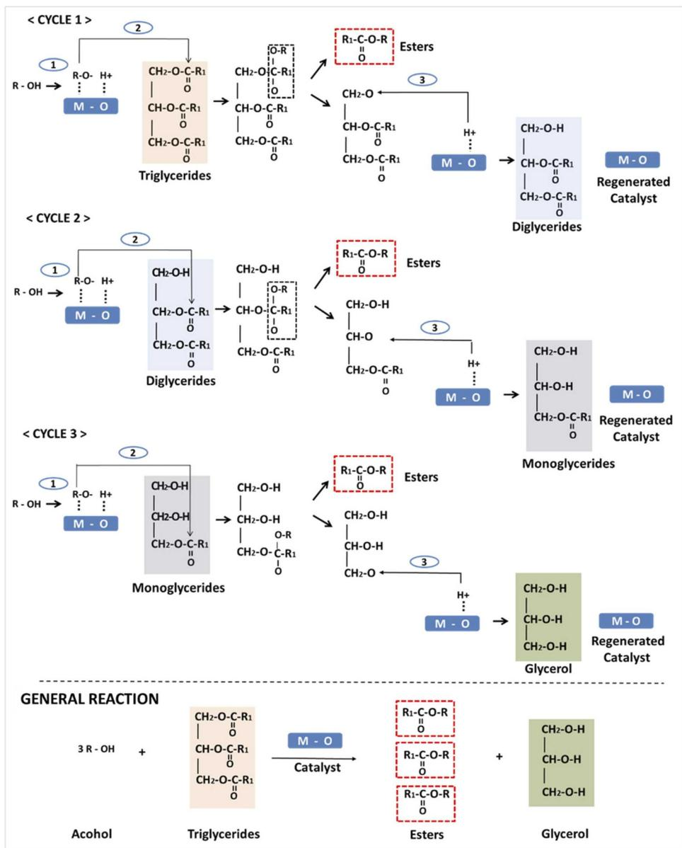
Scheme 1 Mechanism of transesterification.
