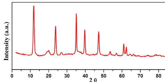
Fig. 3 X-ray diffraction patterns of NiMo/LDH.
