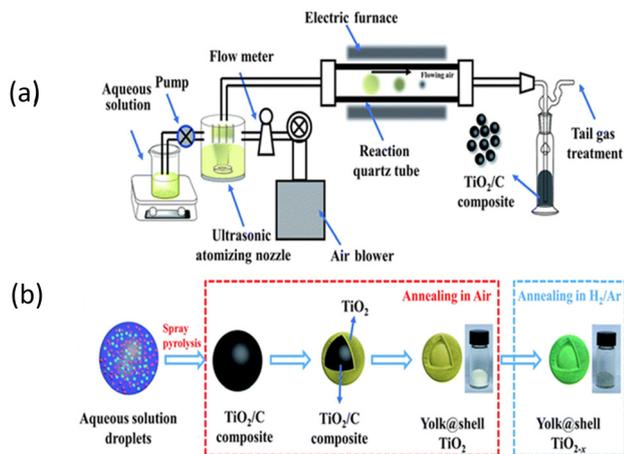
Fig. 4 Schematic diagram of (a) ultrasonic spray pyrolysis process and (b) mechanism of yolk@shell-structured TiO<sub>2-x</sub> prepared using the ultrasonic pyrolysis method. Reprinted with permission from ref. 163. Copyright: 2019, the Royal Society of Chemistry.
