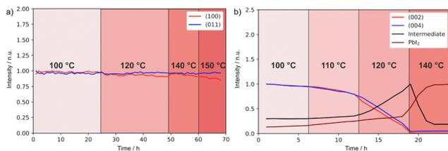
Fig. 4 XRD peak intensity change over time and of (a) (PDMA)PbI<sub>4</sub> sample in the temperature range of 100–150 °C and of (b) (BzA)<sub>2</sub>PbI<sub>4</sub> sample in the temperature range of 100–140 °C in a nitrogen atmosphere. The peak intensities were normalized by taking the initial values at starting temperatures (Fig. S6c, ESI†).
