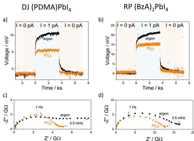
**Fig. 2** Galvanostatic polarization measurements performed on horizontal devices with (a)  $(\text{PDMA})\text{PbI}_4$  and (b)  $(\text{BzA})_2\text{PbI}_4$  thin films in an argon atmosphere and under iodine atmosphere ( $P(\text{I}_2) = 7 \times 10^{-7} \text{ bar}$ ; argon carrier gas) at 60 °C in the dark. Impedance spectra collected under analogous conditions are shown in (c) for the DJ and (d) for the RP film.
