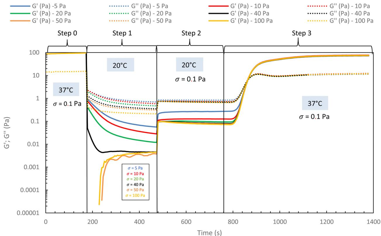
Fig. 7 Rheological injection simulation for HA-*g*-(PiPrOx-co-PBuOx-67/33)-0.10 *via* different stress apply at 20 °C to mimic the injection phenomenon (15 g L<sup>-1</sup> in NaCl 0.15 M).
