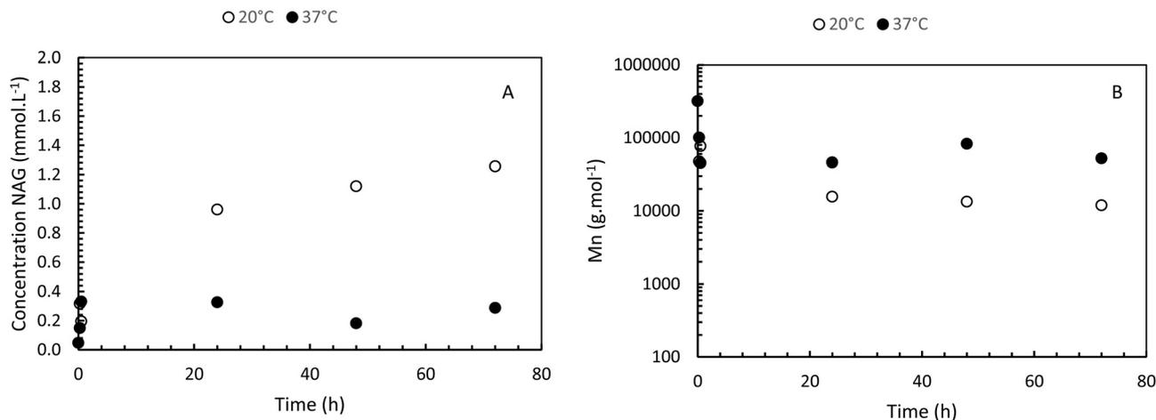
Fig. 5 (A) Enzymatic degradation of HA-g-P(iPrOx-co-BuOx-67/33)-0.10 in presence of hyaluronidase (100  $\mu\text{L}$  at 1 mg mL<sup>-1</sup> for 10 mL hydrogel at 15 g L<sup>-1</sup>) over time at 20 °C and 37 °C. (B) Molar mass evolution of HA-g-P(iPrOx-co-BuOx-67/33)-0.10 over time in presence of hyaluronidase at 20 °C and 37 °C.
