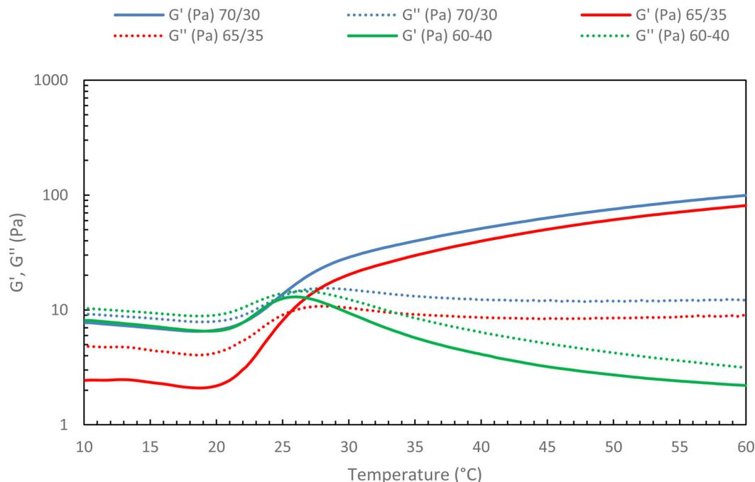
Fig. 11 Rheological ramp of different mixture between HA-*g*-P(iPrOx-co-BuOx-67/33)-0.10 and native HA (15 g L<sup>-1</sup> in NaCl 0.15 M; 0.5 °C min<sup>-1</sup>, 0.1 Pa and 1 Hz).
