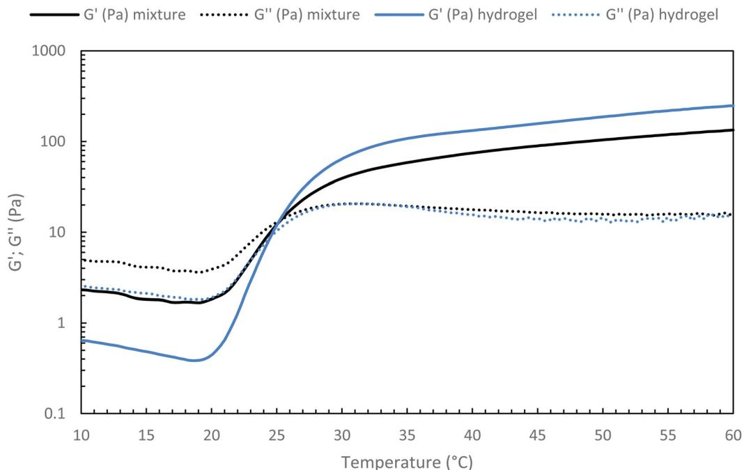
Fig. 10 Temperature ramp for hydrogel alone (HA-*g*-P(iPrOx-co-PBuOx-67/33)-0.10) and hydrogel/HA mixture (75/25 – v/v) at 15 g L<sup>-1</sup> in NaCl 0.15 M (0.1 Pa and 1 Hz; 0.5 °C min<sup>-1</sup>).
