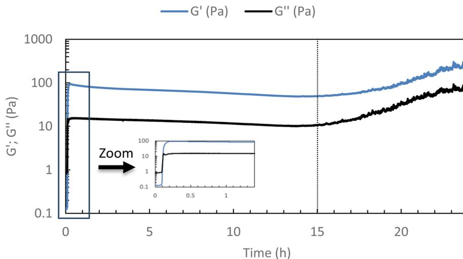
Fig. 3 Stability studies of HA-g-P(iPrOx-co-BuOx-67/33)-0.10 at 37 °C (15 g L<sup>-1</sup> in NaCl 0.15 M) for 24 h (0.1 Pa and 1 Hz).
