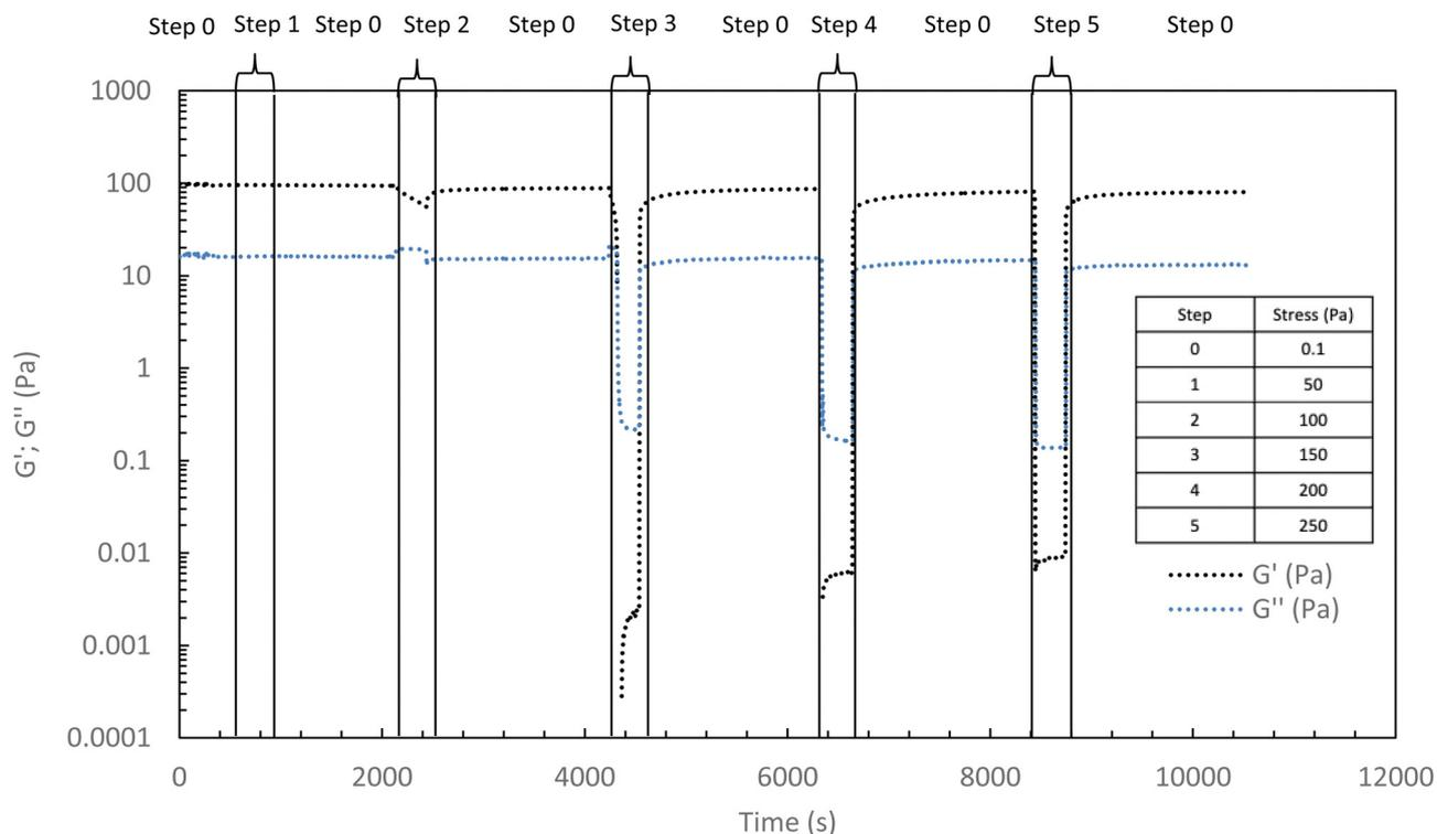
Fig. 9 Elastic and viscous moduli during different stresses applications (ranging from 50 to 250 Pa) to the hydrogel (HA-PiPrOx-co-PBuOx-66/34-0.10,  $15 \text{ g L}^{-1}$  in NaCl 0.15 M) at 37 °C (1 Hz) with a rest time (0.1 Pa, 1 Hz) between stresses.
