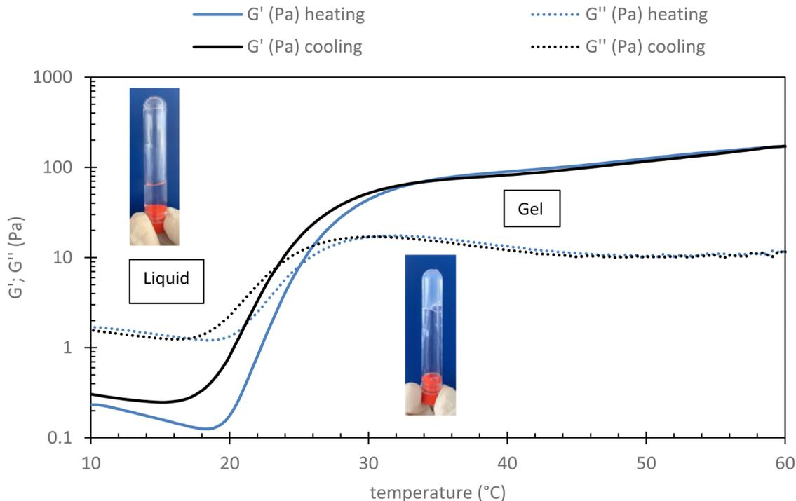
Fig. 2 Evolution of rheological profile of HA-g-P(iPrOx-co-BuOx-67/33)-0.10 0.15 g L<sup>-1</sup> in NaCl 0.15 M in function of temperature (shear stress: 0.1 Pa; frequency: 1 Hz and rate: 0.5 °C min<sup>-1</sup>).
