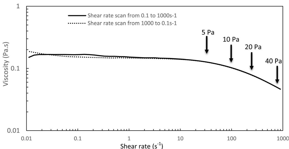
Fig. 6 Flow curve for HA-g-P(iPrOx-co-BuOx-67/33)-0.10 at 20 °C; 15 g L<sup>-1</sup>.
