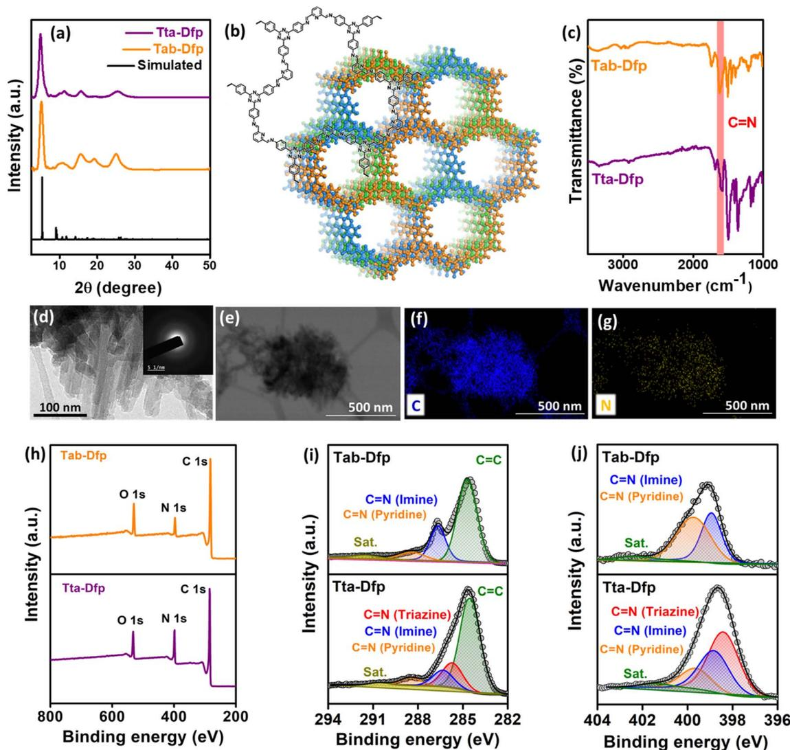
Fig. 1 (a) Experimental and simulated P-XRD patterns of Tta-Dfp and Tab-Dfp,<sup>45</sup> (b) ChemDraw and simulated structures of Tta-Dfp, (c) FT-IR spectra of Tta-Dfp and Tab-Dfp representing the formation of imine linkages, (d) HR-TEM image of Tta-Dfp (inset displaying the SAED pattern), (e–g) TEM-EDS scanned area and dot mapping images showing C and N, (h) XPS survey spectra, and deconvoluted (i) C 1s and (j) N 1s of Tta-Dfp and Tab-Dfp.<sup>45</sup>
