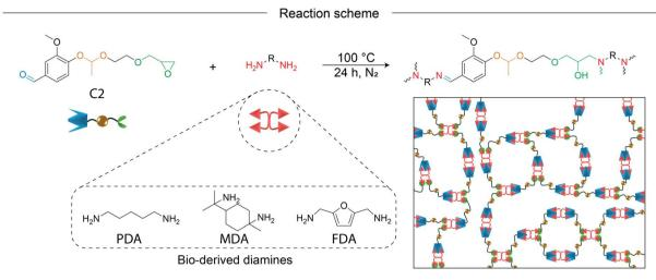
Scheme 1 Synthesis of bio-based, doubly-cleavable epoxy networks
