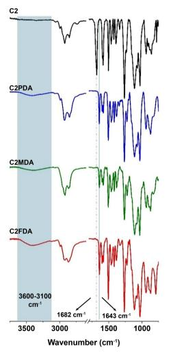
Fig. 1 FTIR spectra of the C2 monomer and the cured networks.
