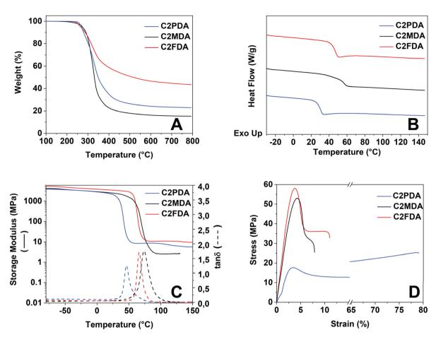
Fig. 2 Thermal, thermomechanical and mechanical characterization of the epoxy networks: TGA (A), DSC (B), DMA (C), tensile tests (D).
