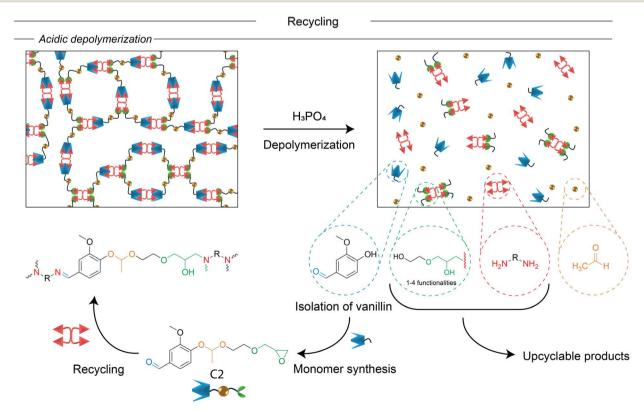
Illustration of the recycling of designed epoxy networks utilizing controlled acidic depolymerization with 1 M H<sub>3</sub>PO<sub>4</sub> solution.
