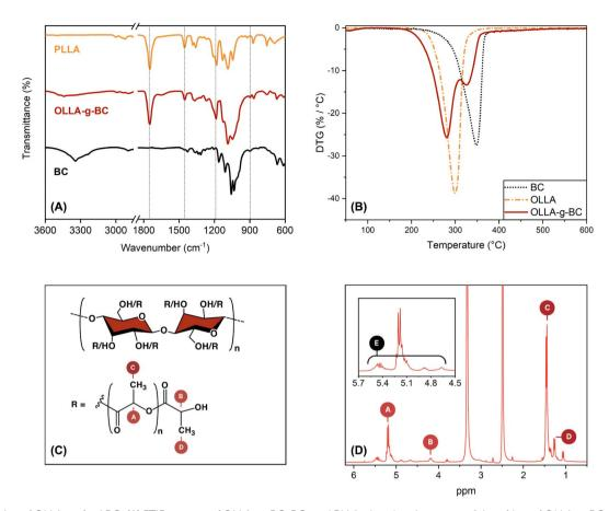
Fig. 2 Analytics of OLLA grafted BC; (A) FTIR spectra of OLLA-g-BC, BC, and PLLA, showing the successful grafting of OLLA to BC nanoparticles. (B) Derivative thermogravimetry data for BC, OLLA, and OLLA-g-BC. (C) Chemical structure of OLLA-g-BC marking the allocation of the NMR peaks in (D) <sup>1</sup>H-NMR spectra of OLLA-g-BC.
