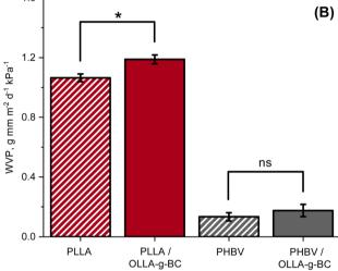
Fig. 5 Comparison of oxygen and water permeabilities: (A) oxygen and (B) water vapor permeability of PLLA, PLLA/OLLA-g-BC, PHBV, and PHBV/OLLA-g-BC.
