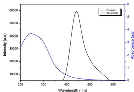
Fig. 3 UV absorbance and fluorescence emission of CD water solution ( $\lambda_{\text{max exc}} = 370$  nm).
