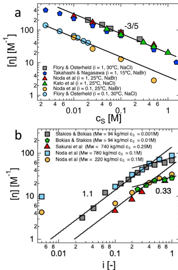
Fig. 22 (a) Dependence of intrinsic viscosity of polyacrylic acid on added salt concentration for  $N \approx 8170$  (see text) for 10% ionisation ( $i = 0.1$ ) and full ionisation ( $i = 1$ ). Power-law of  $-3/5$  is the scaling prediction. (b) Intrinsic viscosity vs. degree of neutralisation  $i$ . Exponents are best fit values. Data are from ref. 195, 537 and 540–543. Results reported by Bokias and Stakios<sup>542</sup> were obtained by isoionic dilution.
