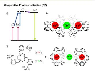
Fig. 7 (a) Cooperative photosensitization (CP) mechanism. (b) bipyridine-based  $Yb_2Tb$  assembly.<sup>41</sup> (c) Stepwise formation of TACN-based  $Yb_2Tb$  assembly.<sup>30</sup>
