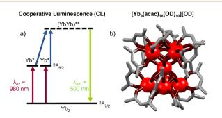
Fig. 10 (a) Energy-level diagram for cooperative luminescence of Yb ions. (b) A  $[Yb_9(acac)_{16}(OD)_{10}][OD]$  system exhibiting CL (ion colors: Yb = red)<sup>67</sup>
