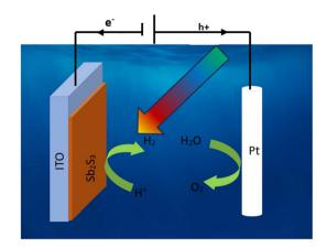
Fig. 17 Schematic mechanism of photoelectrochemical water splitting of  ${\rm Sb_2S_3}$ -based photocathode.
