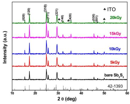
Fig. 6 XRD pattern of Sb<sub>2</sub>S<sub>3</sub> before and after irradiation with various  $\gamma$  radiation doses
