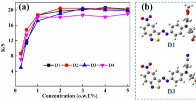
Fig. 5 Build-up curves (a) and optimized geometries (b) of D1–D4.
