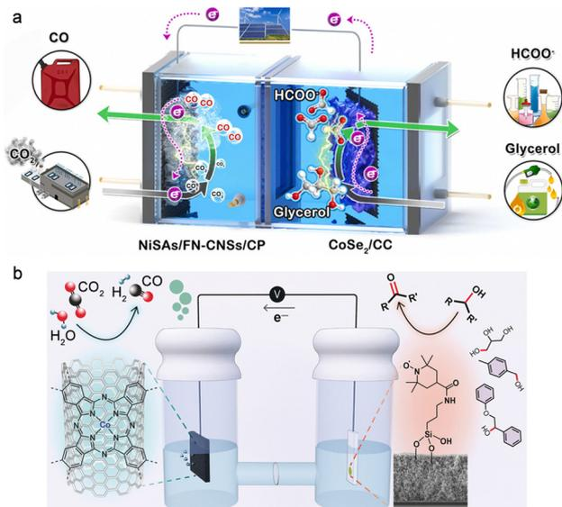
Fig. 5 (a) Schematic illustration of the electrolyser featuring CO<sub>2</sub>RR-to-CO coupled with GOR-to-formate. Reproduced with permission from ref. 40. Copyright 2022, Elsevier Ltd. (b) Coproduction of syngas and glyceraldehyde using the CO<sub>2</sub>RR-GOR couple. Reproduced with permission from ref. 41. Copyright 2020, John Wiley & Sons, Inc.
