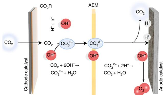
Fig. 9 CO<sub>2</sub> loss via carbonate formation and crossover to the anodic side under alkaline conditions. Reproduced with permission from ref. 65. Copyright 2022, Springer Nature.
