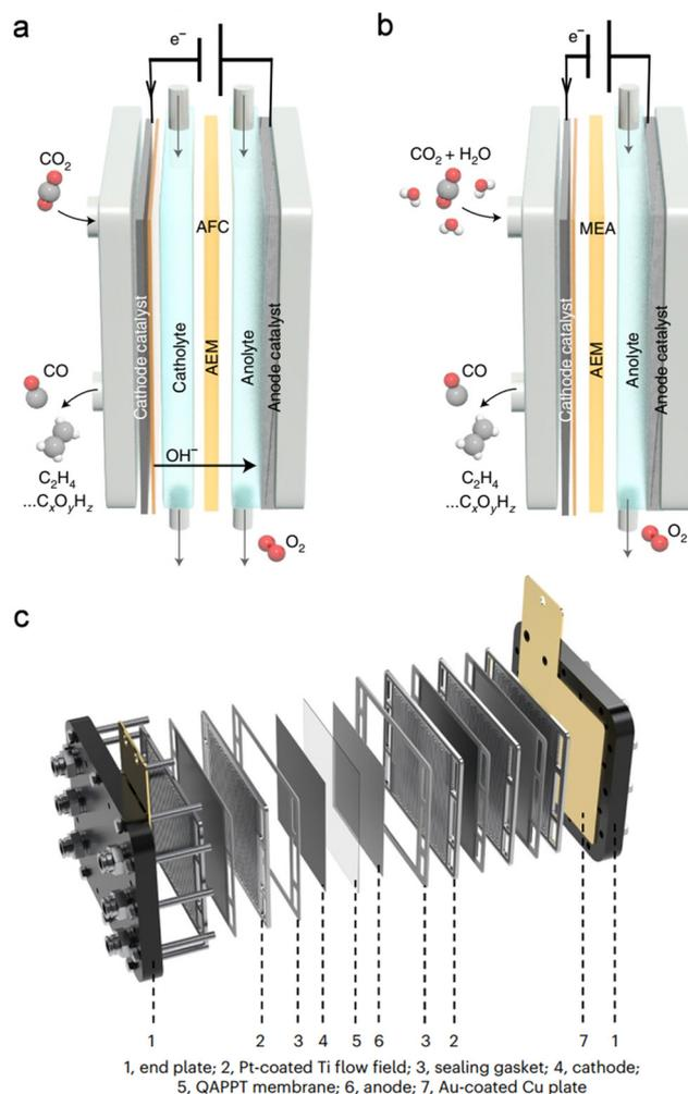
**Fig. 8** Schematic of (a) an alkaline electrolyte flow cell (AFC) and (b) an MEA electrolyser. Reproduced with permission from ref. 65. Copyright 2022, Springer Nature. (c) Scale-up electrolyser stack with four 10 × 10 cm<sup>2</sup> MEAs. Reproduced with permission from ref. 67. Copyright 2023, Springer Nature.
