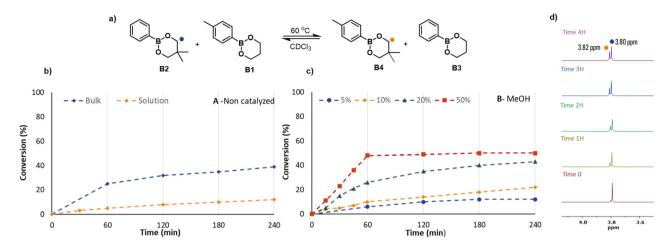
Fig. 4 (a) Experimental kinetics of the reaction between dioxaborinane B2 and B1 at 60 °C for 4 hours. (b) Kinetics of B2 + B1 without catalyst in solution (CDCl<sub>3</sub>) and in bulk. (c) Kinetics of B2 + B1 in solution with 5, 10, 20 and 50 mol% of MeOH with respect to the dioxaborinanes. (d) Time-dependent <sup>1</sup>H-NMR spectra of the bulk kinetic reaction of the two dioxaborinanes.
