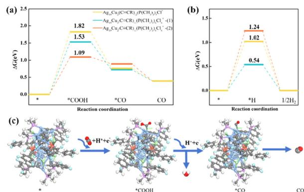
**Fig. 4** Free energy diagrams ( $\Delta G$ ) for  $CO_2$  reduction (a) and hydrogen evolution (b) on  $Ag_{19}Cu_2$  clusters with different ligands removed at zero potential. (c) Schematic presentation of the electrocatalytic  $CO_2$  reduction process on the  $[Ag_{19}Cu_2(C\equiv CR)_{11}(P(CH_3)_3)_6Cl_6]^{+(-2)}$  cluster. Colour legend: Ag, baby blue; Cu, dark orange; C, grey; Cl, light green; F, cyan; P, purple; H, white; O, red.
