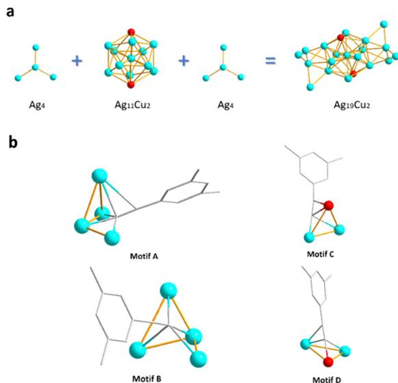
**Fig. 2** (a) The structural anatomy of the  $\text{Ag}_{19}\text{Cu}_2$  core. (b) Four different coordination modes between Ag/Cu and one alkyne molecule. Color legend: red, Cu; blue, Ag; green, Cl; purple, P; laurel green, F; white, H; gray, C.
