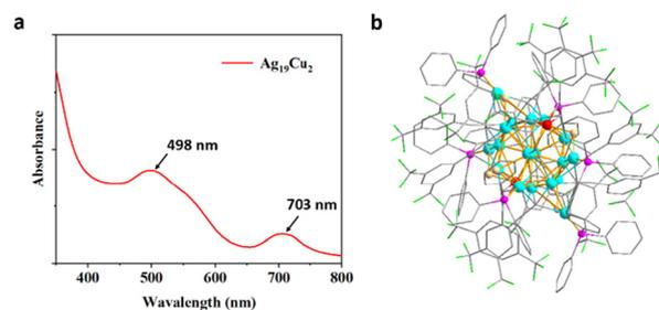
**Fig. 1** (a) Absorbance spectra of the  $\text{Ag}_{19}\text{Cu}_2$  nanocluster in  $\text{CH}_2\text{Cl}_2$ . (b) The overall structure of  $\text{Ag}_{19}\text{Cu}_2$ . Color legend: red, Cu; blue, Ag; green, Cl; purple, P; laurel green, F; white, H; gray, C.
