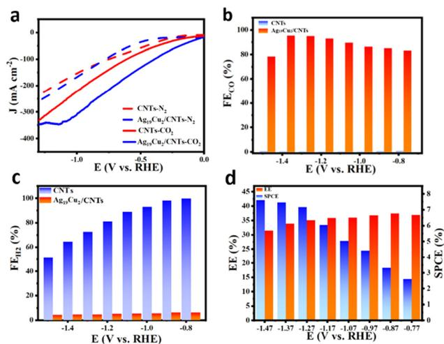
**Fig. 3** (a) Polarization curve of CNTs and  $\text{Ag}_{19}\text{Cu}_2/\text{CNTs}$  in N<sub>2</sub>/CO<sub>2</sub> saturated 1 M KOH. (b) FE<sub>CO</sub> of CNTs and  $\text{Ag}_{19}\text{Cu}_2/\text{CNTs}$ . (c) FE<sub>H<sub>2</sub></sub> of CNTs and  $\text{Ag}_{19}\text{Cu}_2/\text{CNTs}$ . (d) EE and SPCE of the eCO<sub>2</sub>RR.
