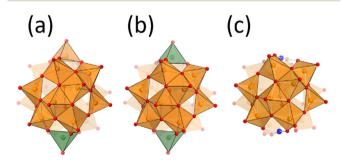
Fig. 1 Anion structures of (a) V18ox, (b) V18, and (c) Cu2V16. Orange and green square pyramids represent V<sup>5+</sup>O<sub>5</sub> and V<sup>4+</sup>O<sub>5</sub>. Red and blue spheres represent oxygen and copper atoms. The deep and pale colours of the V5+O5 units represent front and back sides. Nitrate locates at the centre of the clusters.
