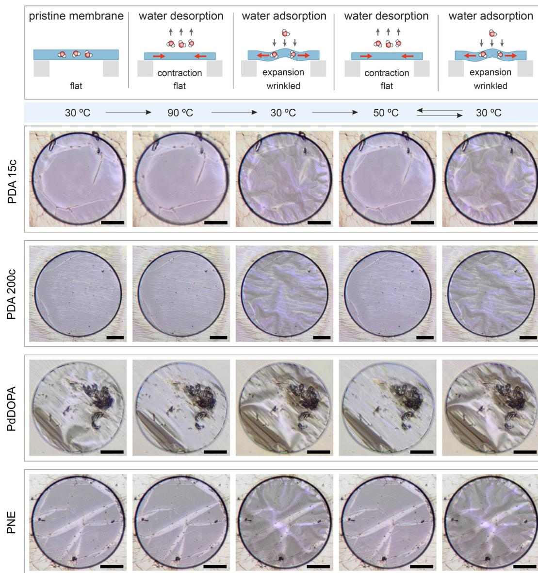
**Fig. 3** Response of the PCA membranes to a uniform thermal stimulus. The left column schematically shows consecutive experiment steps (denoted with black dashed arrows) and a response of the cross-sectioned membrane subjected to global heating. The optical images of the PDA 15c, PDA 200c, PdDOPA, and PNE membranes display their morphology under the selected environmental conditions. The black scale bar is 20  $\mu\text{m}$ .
