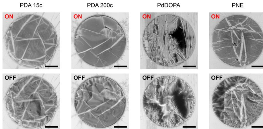
**Fig. 4** (a) Optical images of the various PCA membranes subjected to the red laser light of 20 mW (ON) and the dark conditions (OFF). The black scale bar is 20  $\mu\text{m}$ . To record the photos, a set of polarizers and an optical filter were used to cut off red laser illumination.
