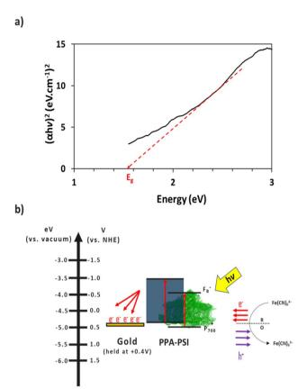
Fig. 8 (a) Tauc plot of PPA. The intersection of the dashed line with the x-axis indicates PPA's band gap. (b) Schematic of the proposed electron transfer mechanism between the redox mediator, the composite film, and the gold substrate, neglecting recombination. Electron movement is represented in red and hole movement is represented in purple
