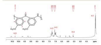
Fig. 2 <sup>1</sup>H NMR spectrum and proposed molecular structure of PPA, as determined by 2D NMR analysis in Fig. S2 and S3.† The molecular structure shows only the benzenoid structures, while the quinoid structure has been omitted for clarity. Hydrogen atoms are enumerated in the molecular structure and their corresponding peaks in the  $^{1}$ H NMR spectrum are labeled in red.
