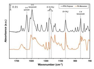
Fig. 1 ATR-FTIR spectra of p-anisidine and PPA with characteristic peaks noted. The spectra are offset vertically for clarity.
