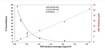
**Fig. 6** Percent light transmittance at *chlorophyll a* absorption wavelengths (440 nm and 675 nm) (left axis) and profilometric film thicknesses (right axis), all with varying PPA surface coverage. The red dotted line represents the linear fit through the film thickness data points. The green and black dotted lines represent the best fit model based on Beer–Lambert law for %T at 440 nm and 675 nm, respectively.
