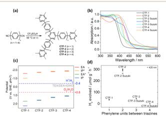
Fig. 14 (a) Synthesis of CTF-n via acid-catalyzed cyclotrimerization. (b) Corresponding absorption spectra. (c) Calculated reducing (EA, IP\*) and oxidizing potentials (IP, EA\*) for CTF-3. (d) Relationship between H<sub>2</sub> yield and number of repeating phenylene units for CTF-n. Reproduced with permission from ref. 115. Copyright 2017, Elsevier.
