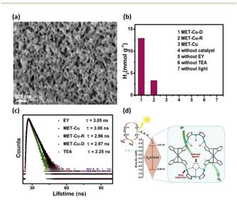
Fig. 5 (a) SEM images of MET-Cu-D and MET-Cu (inset). (b) Results of photocatalytic  $H_2$  production under visible light illumination over the three samples under different conditions. (c) Time-resolved PL spectra of EY in the presence of the three samples. (d) Proposed mechanism of interfacial charge transfer for MET-Cu-D. Reproduced with permission from ref. 42. Copyright 2021, Elsevier.
