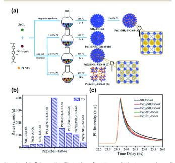
Fig. 11 (a) Schematic illustration for three distinct scenarios of incorporating Pt nanoparticles in NH2-UiO-68. (b) Results of CO production from photocatalytic CO2 reduction under visible light illumination over relevant samples. (c) Time-resolved PL spectra of pristine NH2-UiO-68 and various Pt-incorporated NH2-UiO-68. Excitation and emission wavelength were 360 nm and 475 nm, respectively. Reproduced with permission from ref. 98. Copyright 2016, Wiley.
