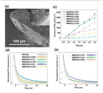
Fig. 1 (a) SEM and (b) HRTEM images for BMOF(Sr)-0.2Fe. (c) Results of photocatalytic NH3 synthesis under white light illumination on various BMOFs samples. (d) Time-resolved PL data of MOF(Sr) and various BMOF(Sr) samples. (e) Time-resolved PL data of BMOF(Sr)-0.2Fe, BMOF(Sr)-0.2Co and BMOF(Sr)-0.2Ba. Reproduced with permission from ref. 37. Copyright 2021, American Chemical Society.
