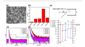
Fig. 6 (a) SEM images of UiO-66-6 and UiO-66-0 (inset). (b) Results of CO production from photocatalytic CO $_2$  production under visible light illumination over various UiO-66-X. (c and d) Time-resolved PL spectra of various UiO-66-X. (e) Proposed mechanism of the energetic state of missing ligands and derived band structure for various UiO-66-X (X = 0, 2, 4, 6, 8). Reproduced with permission from ref. 43. Copyright 2022, American Chemical Society.
