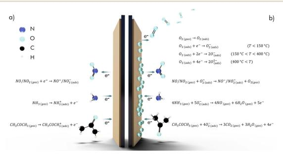
Fig. 3 Reaction equations for NO<sub>2</sub>, NH<sub>3</sub> and acetone on a semiconducting sensor substrate with inert gas (a) and air (b) as support gas. Temperature dependent oxygen adsorption applies to MOx sensors.
