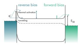
Fig. 2 Typical band diagram of a double-Schottky barrier device in unbiased and biased condition. A potential is applied to the left contact. Electrons flow from left to right; redrawn and adapted, with permission from ref. 39
