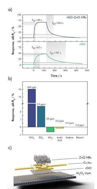
Fig. 9 (a) Dynamic response recovery curves from rGO and the rGO-ZnO NR towards  $NO_2$  at a concentration of 400 ppb, (b) selectivity test using  $NO_2$  (600 ppb),  $SO_2$  (3.5 ppm),  $NH_3$  (35 ppm), acetic acid (3.5 ppm), acetone (3.5 ppm), and ethanol (3.5 ppm); (c) sensor geometry of the stacked rGO-ZnO NR hybrid sensor; redrawn and adapted, with permission from ref. 130.
