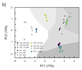
Fig. 16 (a) Feature extraction from the gas response curve (red and blue lines are the exponential fitted curves for the response and recovery regime); (b) decision map for NO<sub>2</sub>, humid air, NH<sub>3</sub>, NO<sub>2</sub> under humid air, and a mixture of  $NO_2$  and  $NH_3$  classified by applying knearest neighbor (kNN) to the PCA model with k = 5; redrawn and adapted from ref. 164.
