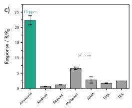
Fig. 12 Hybrid NFI-rGO sensing performance (a) relative response variation as a function of frequency for NH<sub>3</sub> concentrations from 0-60 ppm; (b) dynamic response-recovery curve for exposure to 60 ppm of NH<sub>3</sub>; (c) cross-sensitivity between NH<sub>3</sub> (15 ppm), acetone, ethanol, methanol, monomethylamine (MMA), trimethylamine (TMA) and triethylamine (TEA) (150 ppm); redrawn and adapted, with permission from ref. 146
