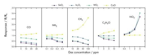
Fig. 15 Signal responses and sample variations of  $SnO_2$ ,  $In_2O_3$ ,  $WO_3$  and CuO towards CO,  $NH_3$ ,  $CH_4$ , acetone and  $NO_2$ ; reprinted (adapted) with permission from ref. 162. Copyright 2022 American Chemical Society.
