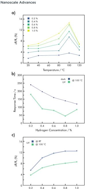
Fig. 11 Hybrid Pd/rGO sensing performance (a) temperaturedependent responses towards H<sub>2</sub> at different concentrations; (b) effect of UV-illumination on response times as a function of H<sub>2</sub>concentration at 100 °C; (c) signal responses under UV-illumination at RT and 100 °C as a function of H<sub>2</sub>-concentration; redrawn with data from ref. 82.
