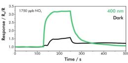
Fig. 10 Sensing mechanism and dynamic response-recovery curves of GTiO<sub>2</sub>S towards 1750 ppb of NO<sub>2</sub> in dark and illuminated operating mode; redrawn and adapted from ref. 138.
